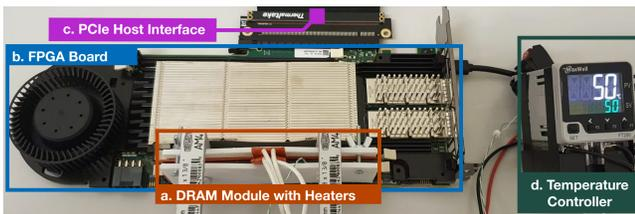
**Fig. 2: SoftMC Infrastructure:** (a) DRAM module under test clamped with heater pads, (b) Xilinx Alveo U200 FPGA board [161], programmed with a DDR4 version of SoftMC [40], (c) PCIe connection to the host machine, and (d) temperature controller.
